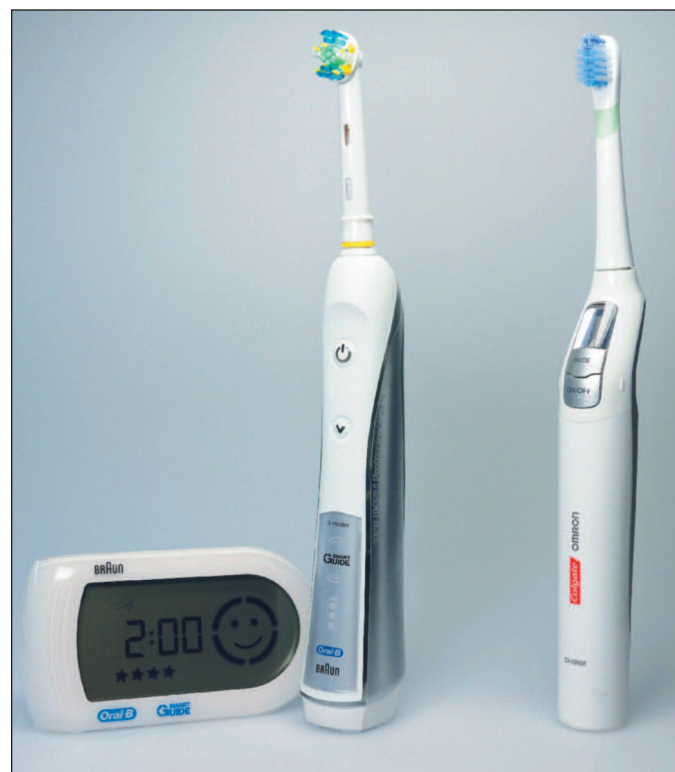
Figure 1. The Oral-B Triumph with SmartGuide and Floss Action brush head (marketed in the US as the Oral-B Professional Care SmartSeries 5000 [D34]) oscillating-rotating brush, and the Colgate ProClinical A1500 sonic brush with Triple Clean brush head.
